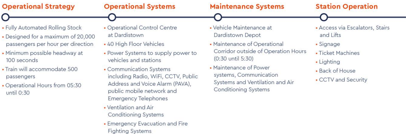
Diagram 1.3: Summary of Key Activities during the Operation Phase of the Proposed Project
